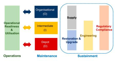
**Figure 1.** The different elements of a maintenance and sustainment (technical support) system for military aircraft and their interactions with operational readiness and utilisation.
