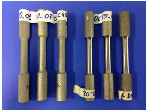
**Figure 3.** Three as built (on the left side) and three machined specimens after EBM process (on the right side).
