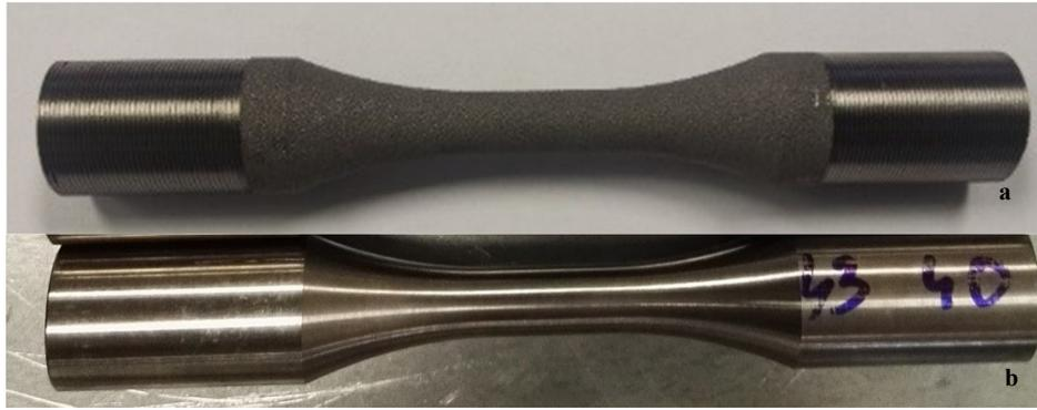
**Figure 6.** (a) Photo of as built specimen; (b) photo of machined specimen.
