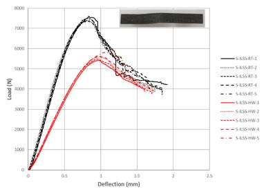
Figure 8. Effect of aging on load-deflection curves measured in ILSS test.
