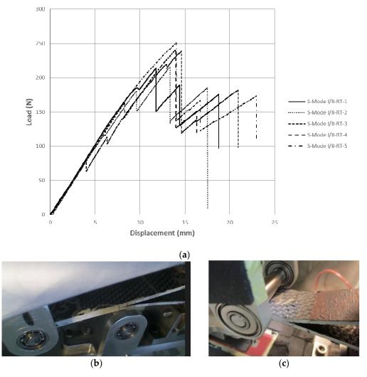
**Figure 12.** Mode II fracture test: (**a**) measured and predicted load vs opening displacement data RT specimens; (**b**) typical deformed shape during RT test; (**c**) failure mode at root of upper face during HW test.
