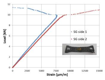
**Figure 4.** Compression test for warp-directional laminate: typical measured load vs longitudinal strain data and typical failure mode (SG: strain gauge).
