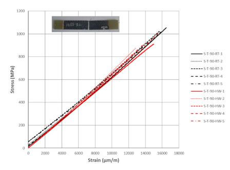
Figure 3. Static tension for weft-directional laminate: stress-strain data and characteristic failure mode.
