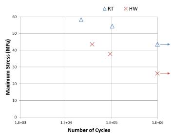
**Figure 9.** Effect of aging on fatigue interlaminar shear strength. Arrows to the right indicate that no failure has occurred.
