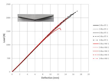
Figure 6. Static flexure: load-deflection data and typical failure mode.
