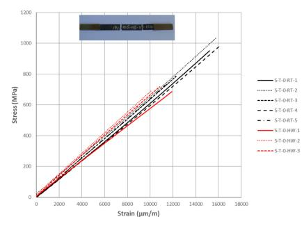
**Figure 2.** Static tension of warp-directional laminate: stress vs strain data and characteristic failure mode at RT. The description of tests follows a custom naming convention: S—static, T—tension, 0—warp direction, RT—room temperature test, HW—hot wet test, last digit—specimen number.
