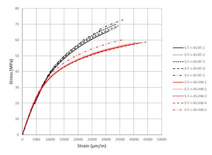
Figure 7. Effect of aging on stress-strain curves of in-plane shear strength (IPSS) test.
