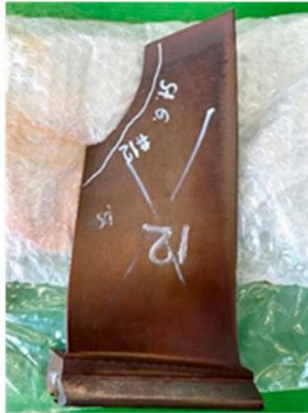
**Figure 1.** An example of compressor blade fracture.
