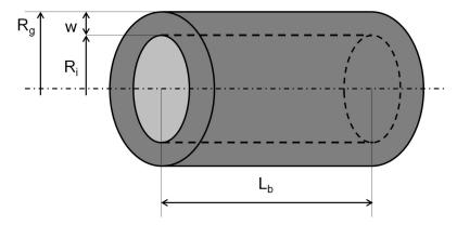
Figure 1. Schematic of the grain geometry.
