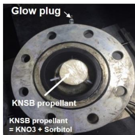
Figure 9. KNSB igniter mounted in pre-chamber.
