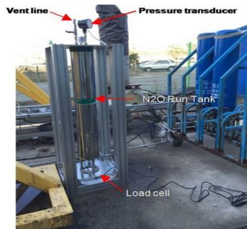
Figure 5. Oxidizer run tank and mass flow measurement.
