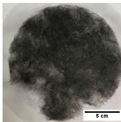
Figure 1. One layer of Sample 2 with 75% rCF and 25% flax.
