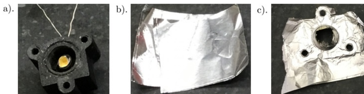
Figure 4. (a) Inside the chamber, the connected heating element holding the aluminum foil cup before enclosure; (b) the aluminum 8011 alloy rupture disc before firing; and (c) the aluminum 8011 alloy rupture disc after firing.
