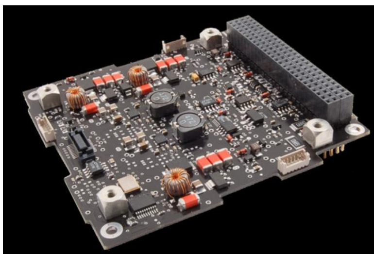
Figure 10. PMAD Developed by Clyde Space Industries [25].
