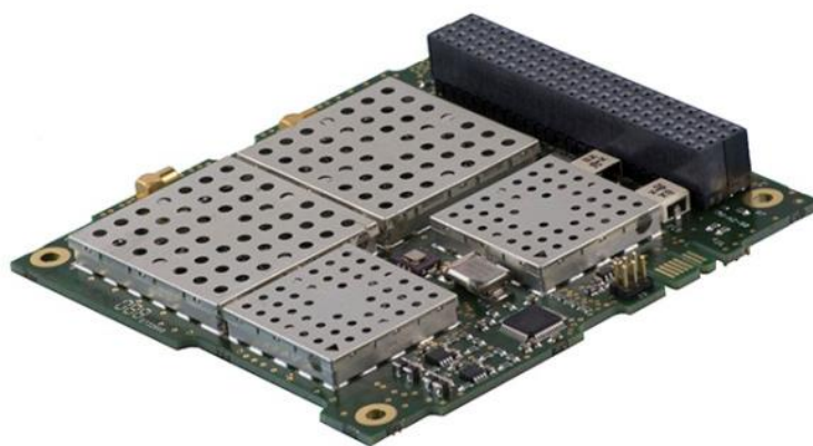
Figure 30. UHF Downlink/VHF Uplink Transceiver [47].
