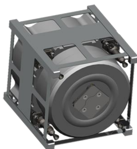
Figure 12. CHAMPS 1U Hydrazine Propulsion System [32].
