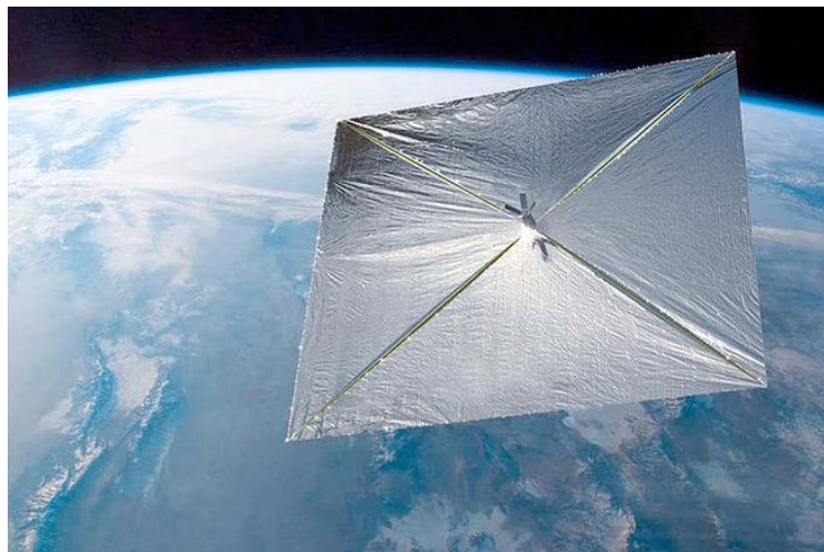
Figure 23. Solar Sail Attached to a 3U CubeSat in Orbit [40].
