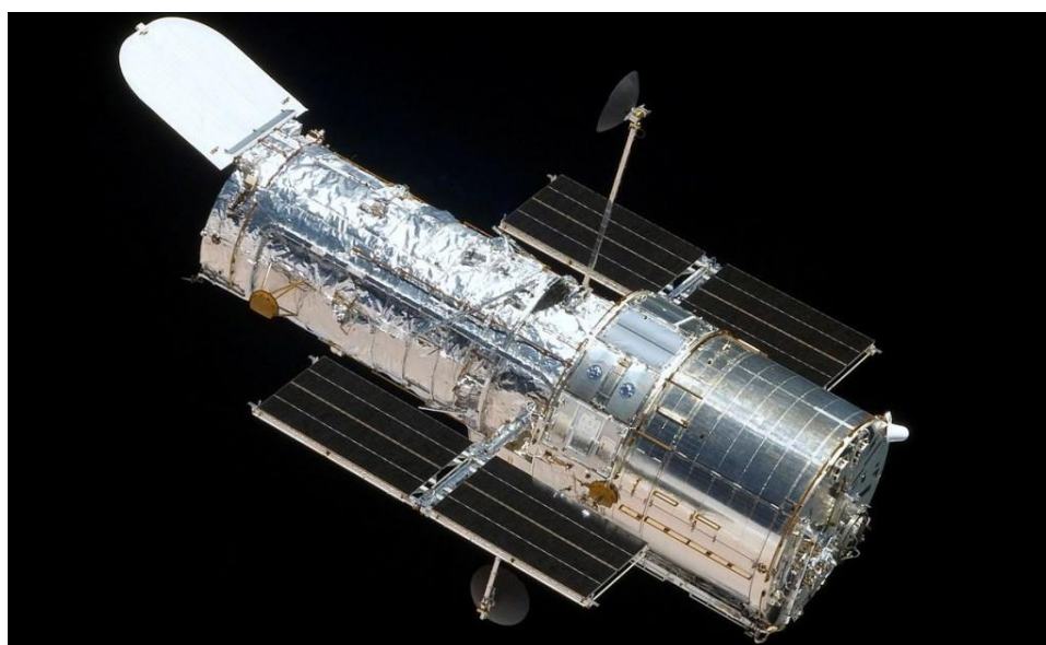
Figure 25. MLI Blanket Incorporated Satellite in Orbit [41].
