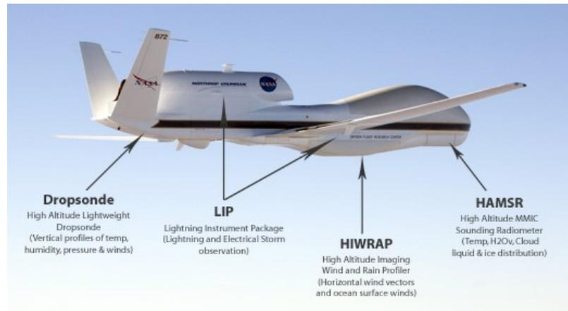
**Figure 1.** NASA's Global Hawk platform and payload as configured for the GRIP mission (courtesy of NASA ESPO).
