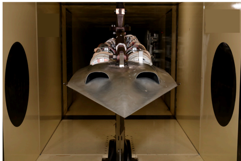
Figure 2. Photograph of the inlet model installed in the test section of the 1.2 m transonic wind tunnel.
