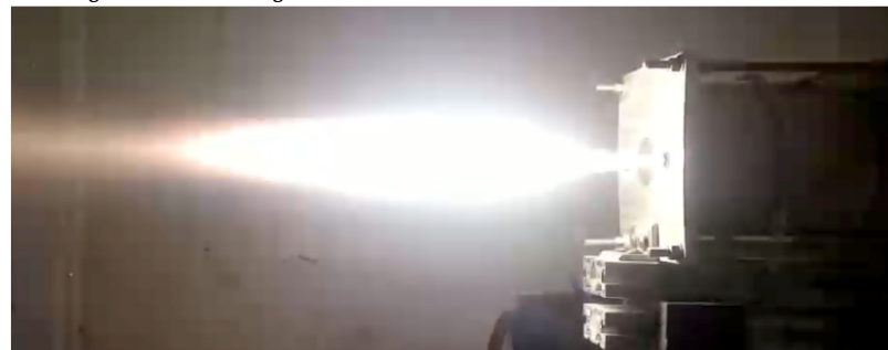
Figure 8. Exhaust plume images for low-pressure (Figure 8) and high-pressure (Figure 9) Nytrox ignition tests.
