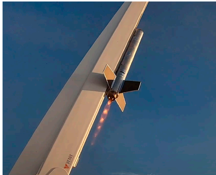
Figure 8. Flight test of a rotating detonation rocket engine (RDRE) demonstrator developed by Venus Aerospace during a successful launch campaign (frame extracted from flight video, 2025).
