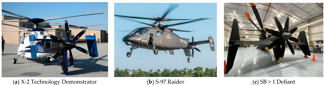
Figure 1. The compound high-speed helicopter with a pusher propeller.
