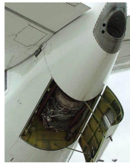
Figure 5. B747-8 Auxiliary Power Unit (APU).
