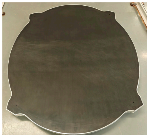
Figure 21. Engineering prototype of the carbon fiber honeycomb core reflector.
