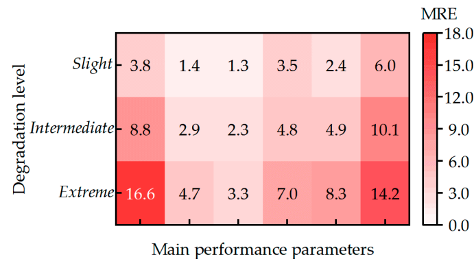
Figure 22. Heatmap of MRE of main performance parameters for regular N-R method and Jacobi Invers N-R method under three degradation levels.
