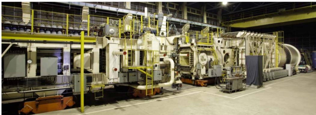
Figure 1. INCAS trisonic wind tunnel [23].
