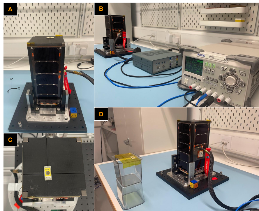
Figure 2. (A) EIRSAT-1, including co-ordinate system, on vertical integration stand for energy calibration measurements with a source positioned on the +Z endcap. (B) GSE for measurements; on the left is the FM, in the centre is the UIU and on the right is the PSU powering the spacecraft. (C) Source positioned on the +Z endcap on cross-hairs marking the centre of the \text{CeBr}_3 crystal. (D) Position of source 6 in Table 2, the source is centred on X of the crystal, 222 mm from the +Y face and 119 mm from the -Z face.
