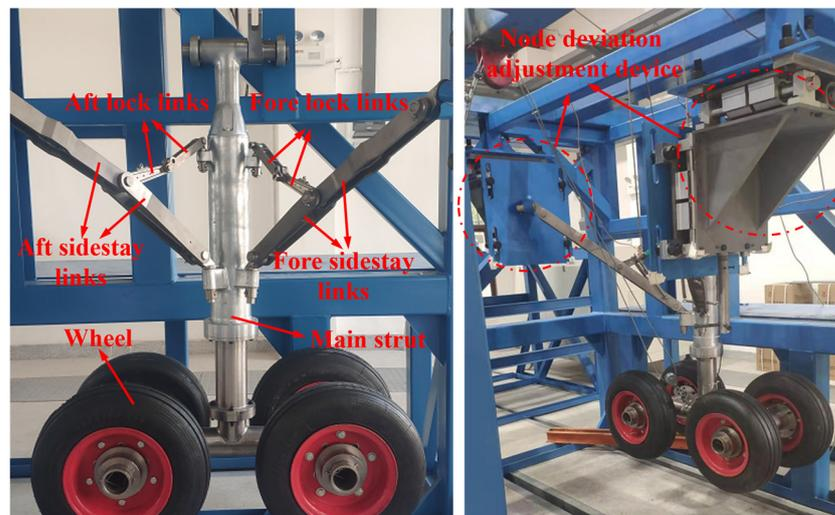
Figure 7. Physical schematic diagram of DSS landing gear test platform.
