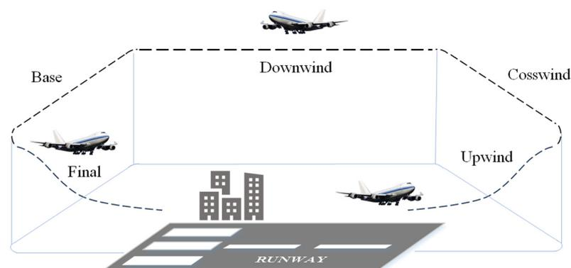
**Figure 2.** Schematic of an airfield traffic pattern.
