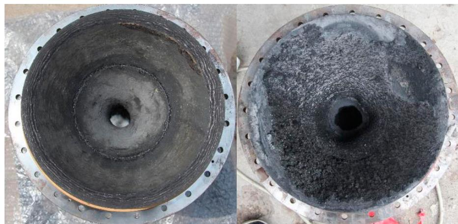
**Figure 16.** The changes in the motor nozzle before and after the 200-s firing test.
