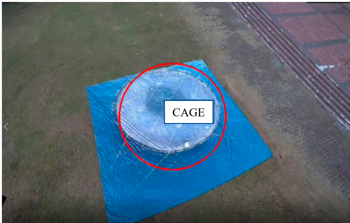
Figure 33. Net cage recognition by the camera on the UAV, the red circle is the center mask of the UAV's camera.
