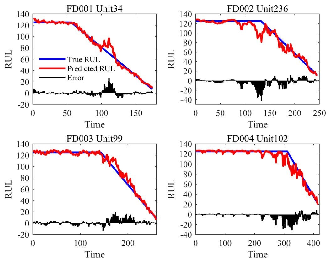
**Figure 5.** Four examples of predicted RUL in the testing set.
