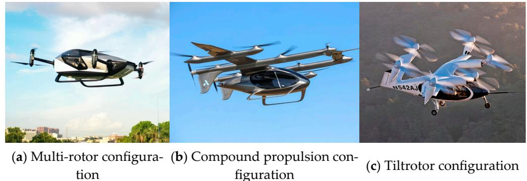
**Figure 1.** Three different configurations of eVTOL.
