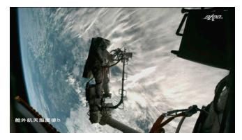
Figure 11. A manipulator was transporting an astronaut and related operation devices.
