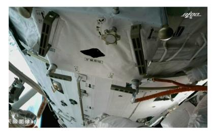
Figure 34. After the installation of the expansion of the extravehicular pump package.
