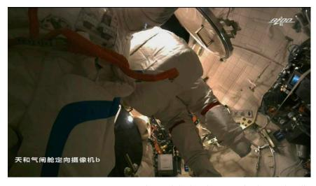
Figure 7. An astronaut was opening the module door by using the driving handle.
