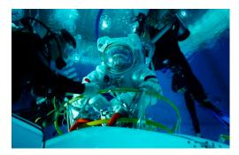
Figure 31. Verification for the exit of astronauts from the airlock under water.
