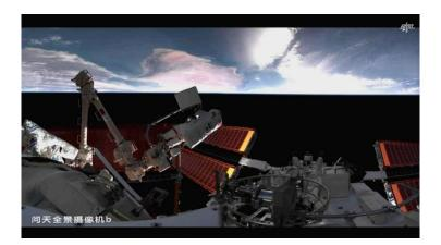
Figure 14. An astronaut was working with the joint help of the manipulators.
