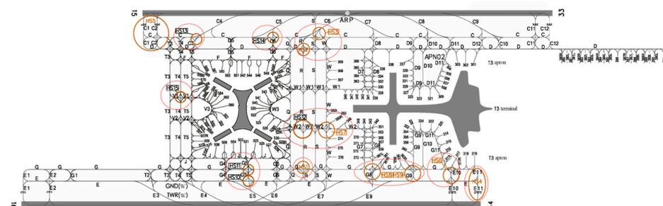
Figure 23. Identification of risk hotspot areas in scene operations based on simulation models and risk assessment.
