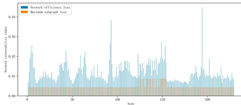
**Figure 19.** Distribution of vulnerability indicators for various nodes at Shenzhen Bao’an Airport.
