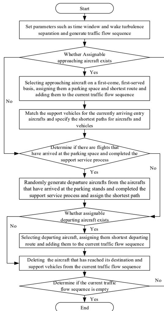
Figure 3. Overall process of airport surface traffic operation simulation.
