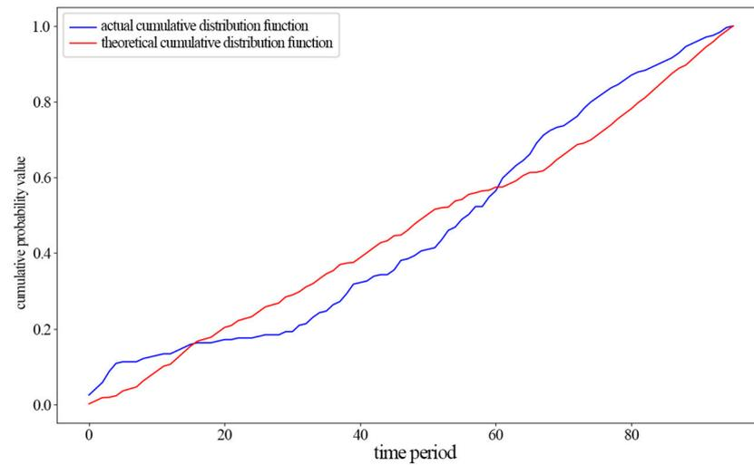
**Figure 8.** Comparison chart of arrival traffic flow cumulative distribution functions.
