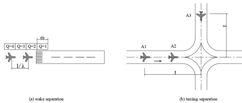
Figure 2. Scene traffic flow conflict allocation rules based on first-come-first-served principle.
