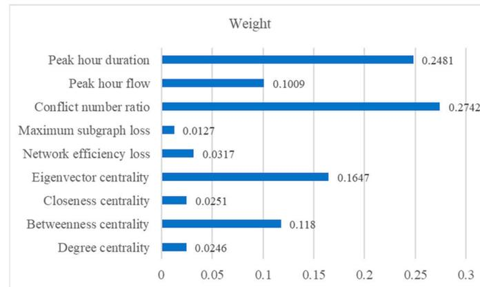
**Figure 20.** Weighting of risk assessment indicators for mixed traffic flow operations in the scene.
