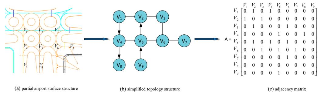
**Figure 1.** The process of modeling the physical structure and topology of the scene.
