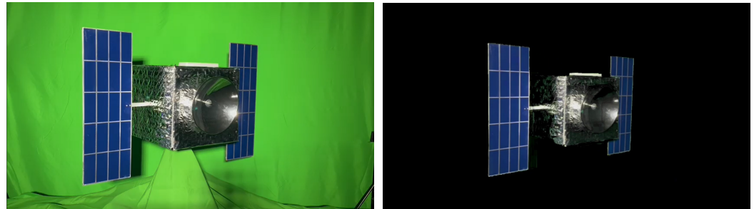
Figure 3. Satellite mock-up with green screen (left) and after chroma key compositing post-processing (right).
