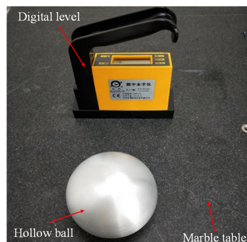
Figure 19. Static balance test of a spherical shell.
