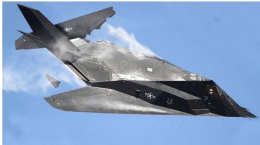
Figure 2. F-117 crash due to elevon flutter ( https://crewdaily.com/well-known-jet-ejections-of-the-aviation-history-part-1/ , accessed on 22 December 2023).
