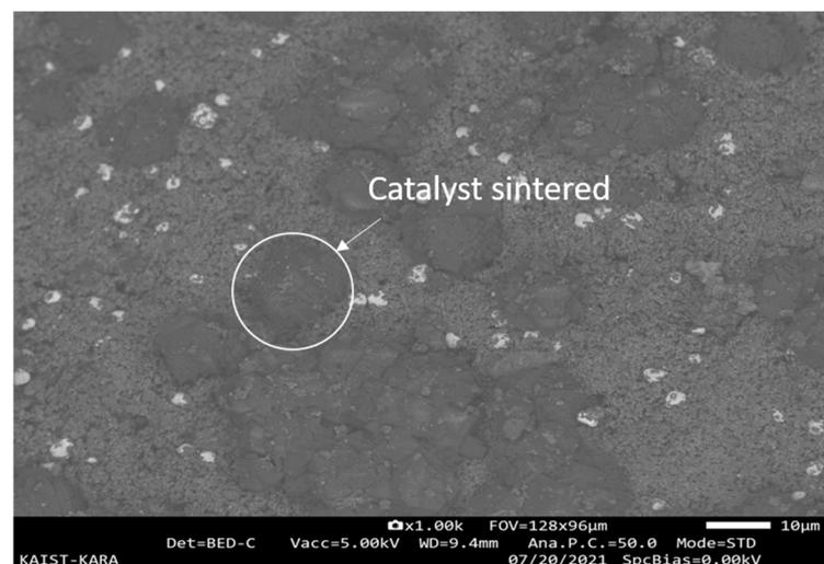
**Figure 16.** SEM image of the Pt-LHA catalyst after the Type-3 reactor test.
