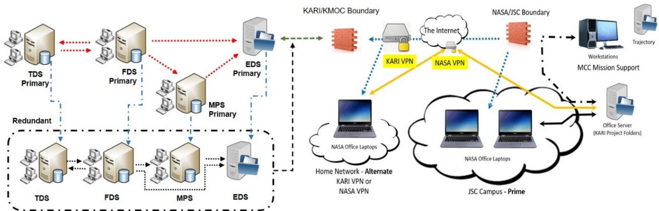
**Figure 5.** Top-level interface architecture between KMOC and MCC.
