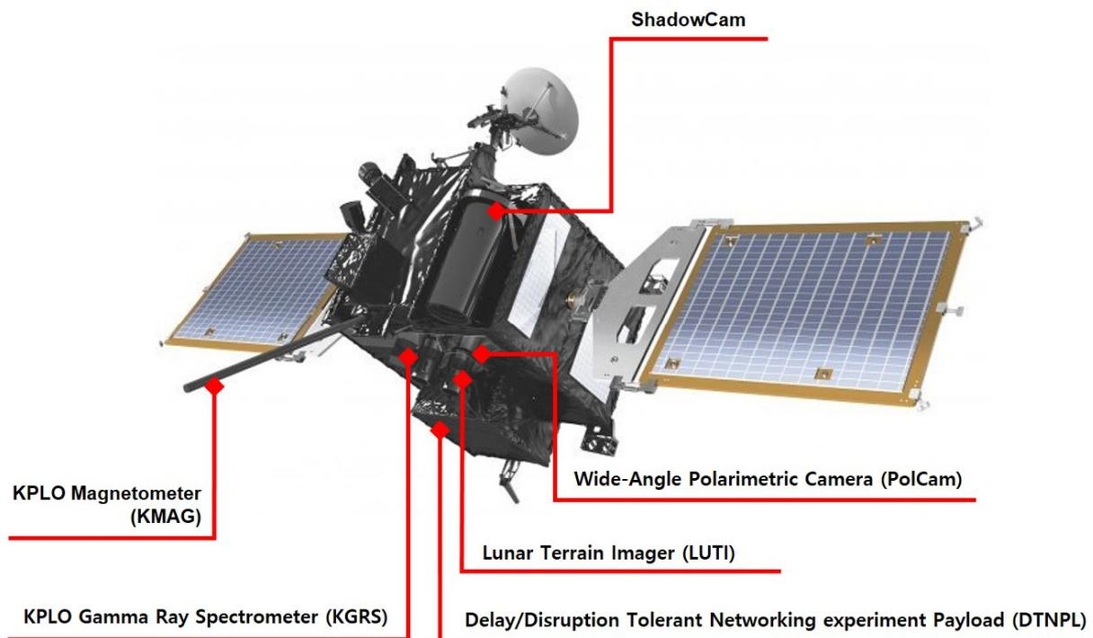
**Figure 1.** KPLO in-flight configuration with location of payloads.
