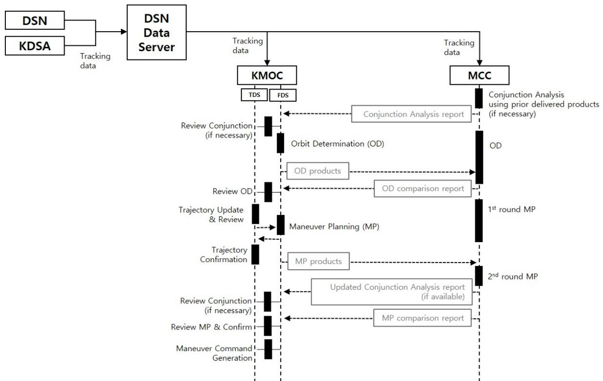
**Figure 4.** Top-level FD joint operation flow between KMOC and MCC.
