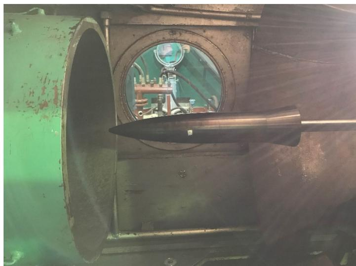
**Figure 21.** Photographs of the experimental model installed in the wind tunnel (FL-31).
