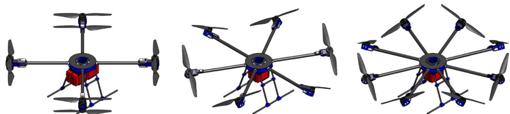
Figure 17. CAD models of non-conventional modular platform configurations (CX8, PTX6, PTX8).
