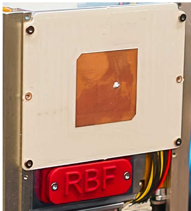
Figure 14. In-house developed circularly polarized S-band patch antenna.
