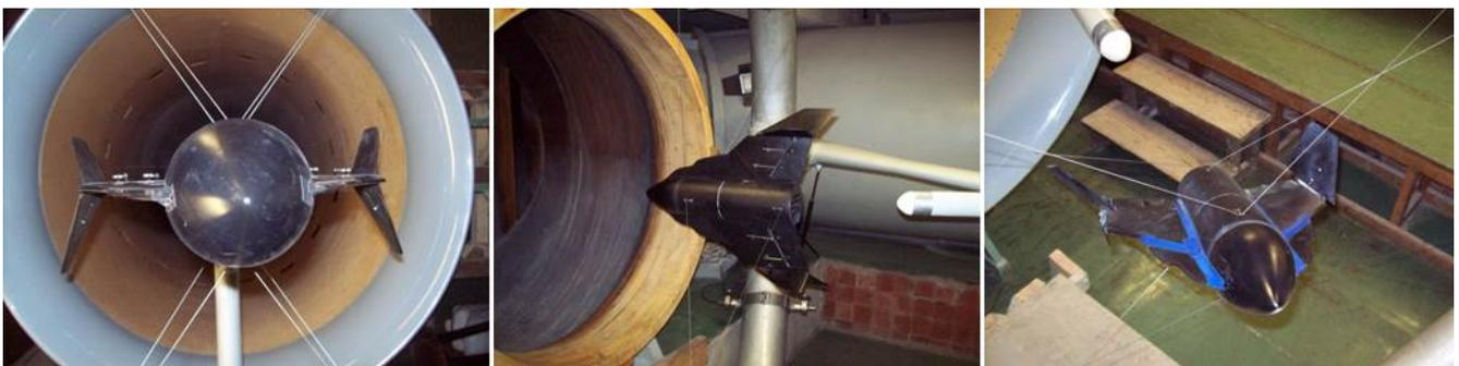
**Figure 6.** Models of the rocket plane during the wind tunnel campaign (at right: the model with deflected side plates).
