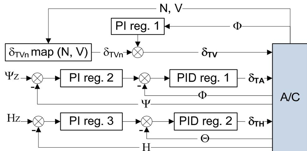
Figure 5. Automatic 3D aircraft stabilisation system.
