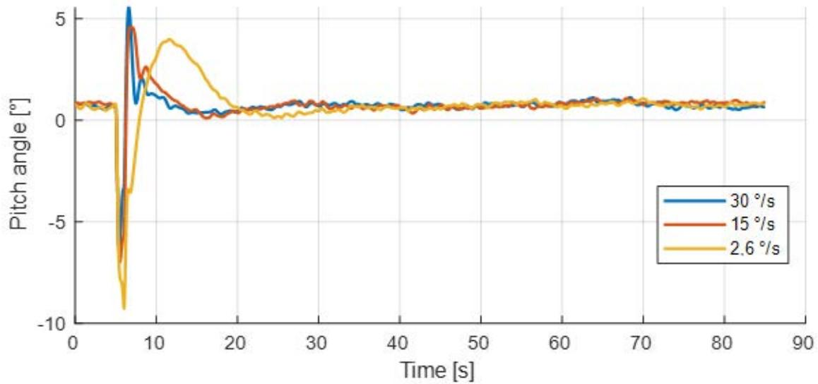
Figure 9. Pitch angle stabilisation after disturbance in the longitudinal channel.
