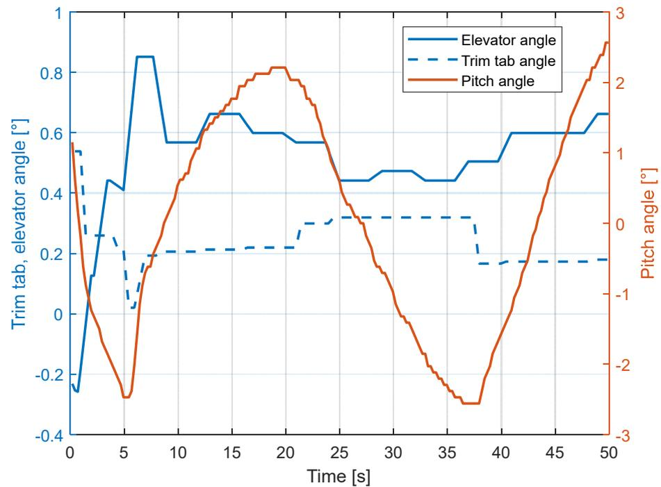
**Figure 3.** Flight test results during the trim-tab-only manually controlled flight—level cruise flight.
