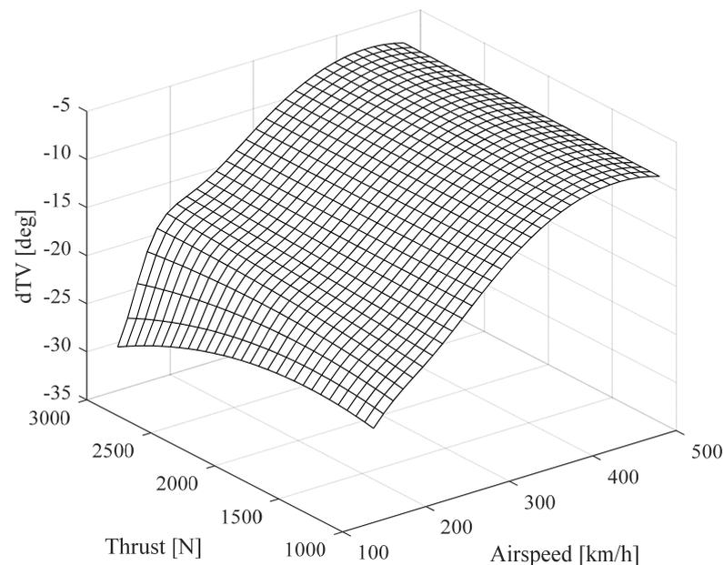
**Figure 6.** Relation between rudder trim tab deflection compensating slipstream effect, thrust and airspeed.
