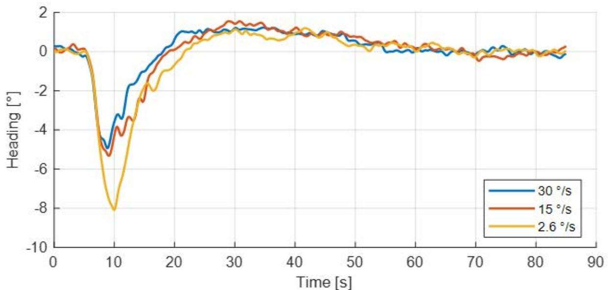
**Figure 11.** Heading stabilisation after disturbance in the lateral channel.
