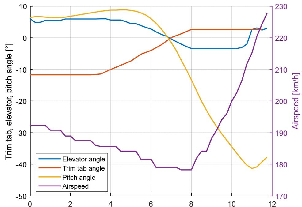
Figure 4. Flight test results of elevator trimmer movement to an extreme position.
