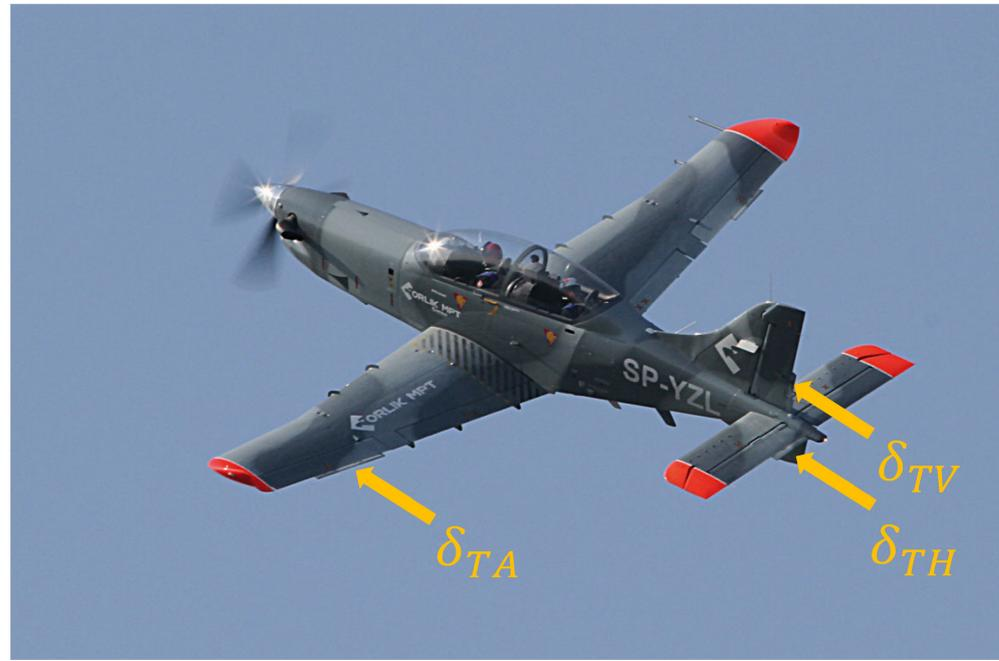
**Figure 1.** Trim tab location on PZL-130 Orlik aircraft.
