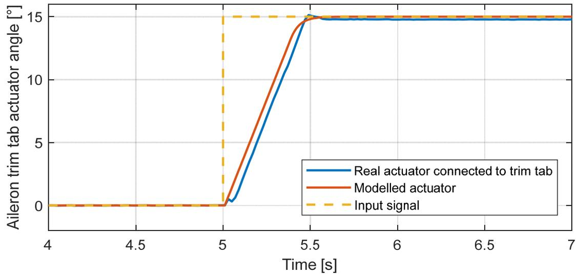
**Figure 7.** Comparison of the genuine actuator and its model response.
