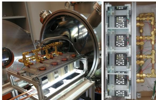
**Figure 5.** Left: SoSi in front of vacuum chamber; right: Four LED clusters and light guides; liquid cooling system for the LEDs.
