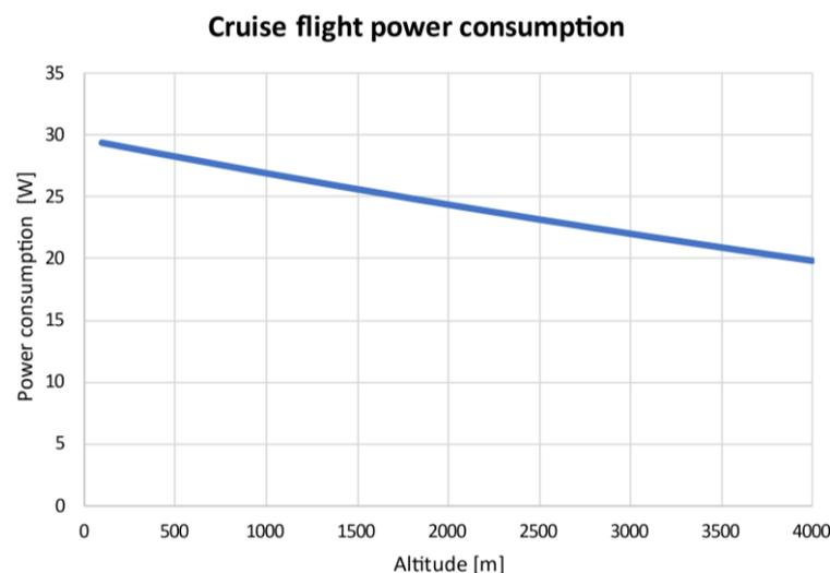
**Figure 9.** Power consumption during cruising for different altitudes.
