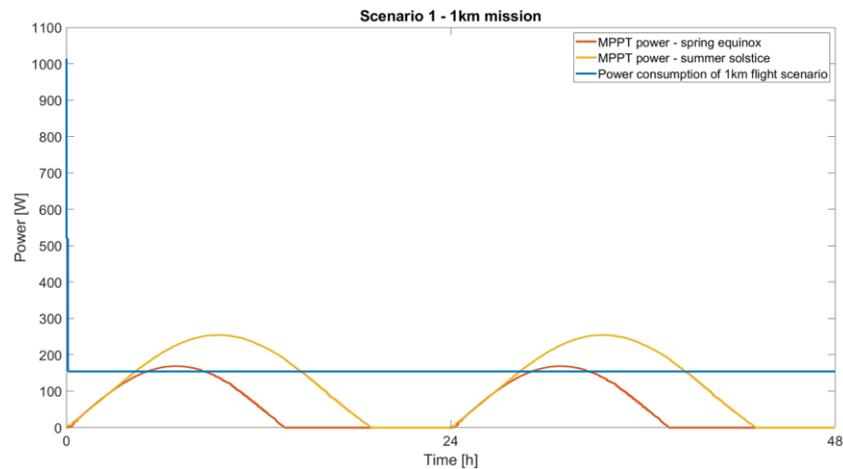
**Figure 11.** Power consumption and MPPT power produced by solar cells for 1st scenario.
