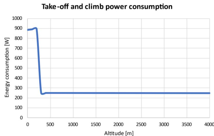
**Figure 8.** Energy consumption during take-off and climbing.
