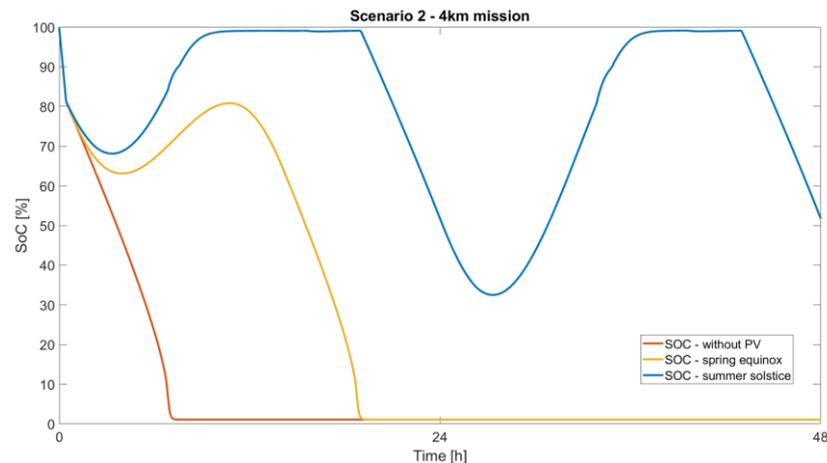
**Figure 12.** State of Charge of the battery during the continuous flight at 4 km.
