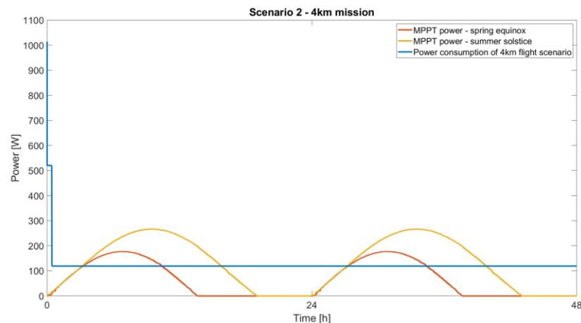
**Figure 13.** Power consumption and MPPT power produced by solar cells for the second scenario.
