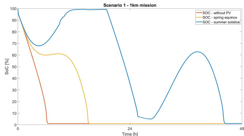
**Figure 10.** State of charge of the battery during the continuous flight at 1 km.
