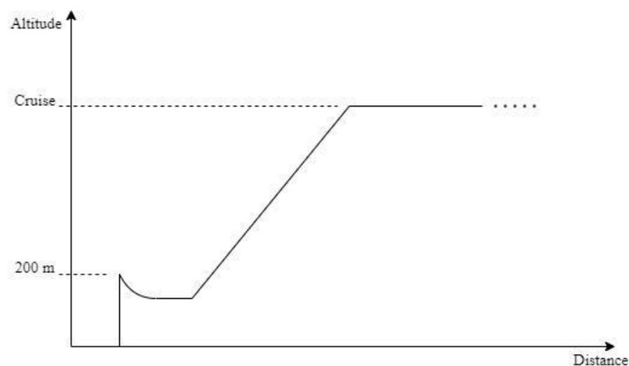
**Figure 2.** A diagram of the vertical take-off and the further climbing as fixed-wing UAV until the cruise altitude.
