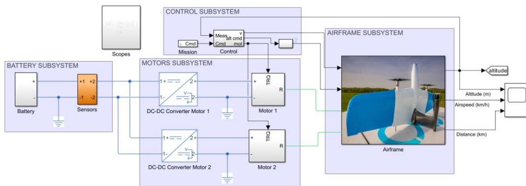
Figure 4. Model for vertical flight simulation.
