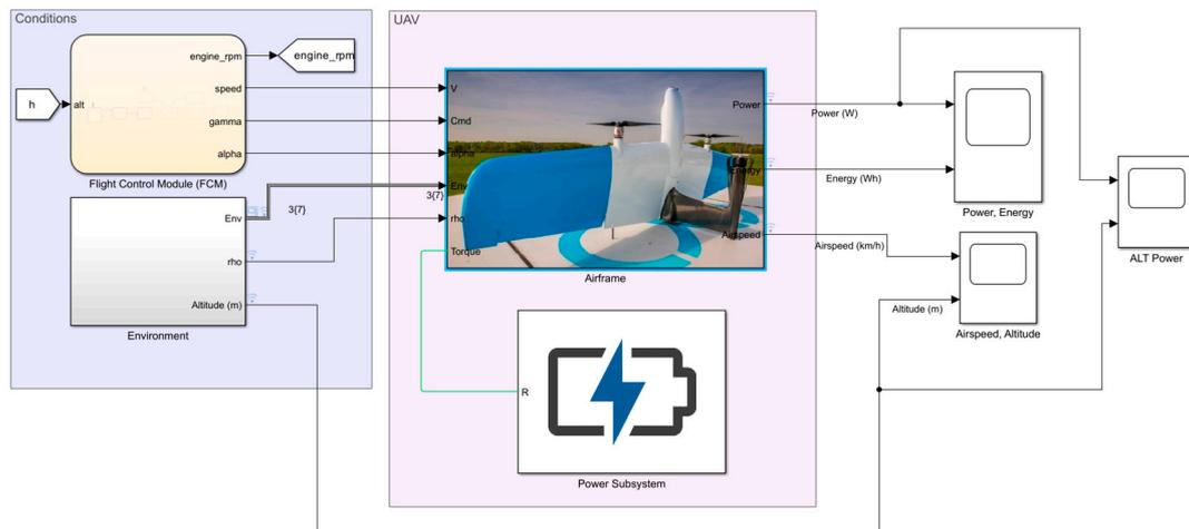
Figure 5. Model for fixed-wing UAV flight simulation.
