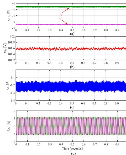
**Figure 26.** Experimental results of steady-state values for generating mode at speed 1000 rpm: (a)  $dq$  voltages references sent to PWM modulator, (b) DC current, (c) DC bus voltage, (d) AC currents.
