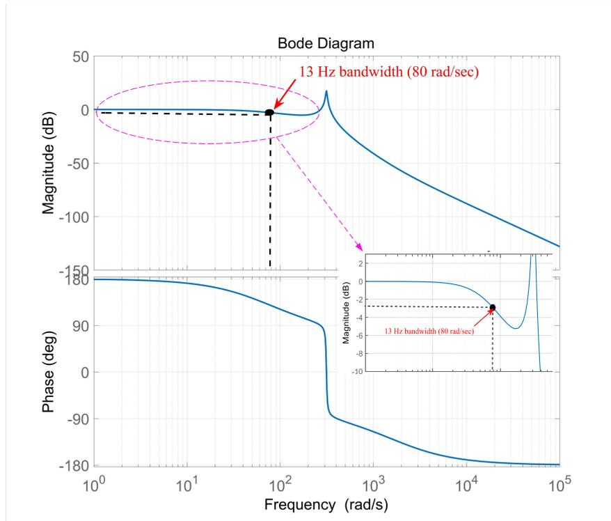
**Figure 8.** Closed-loop plant frequency response at speed 760 rpm and 25% loading for starter mode.
