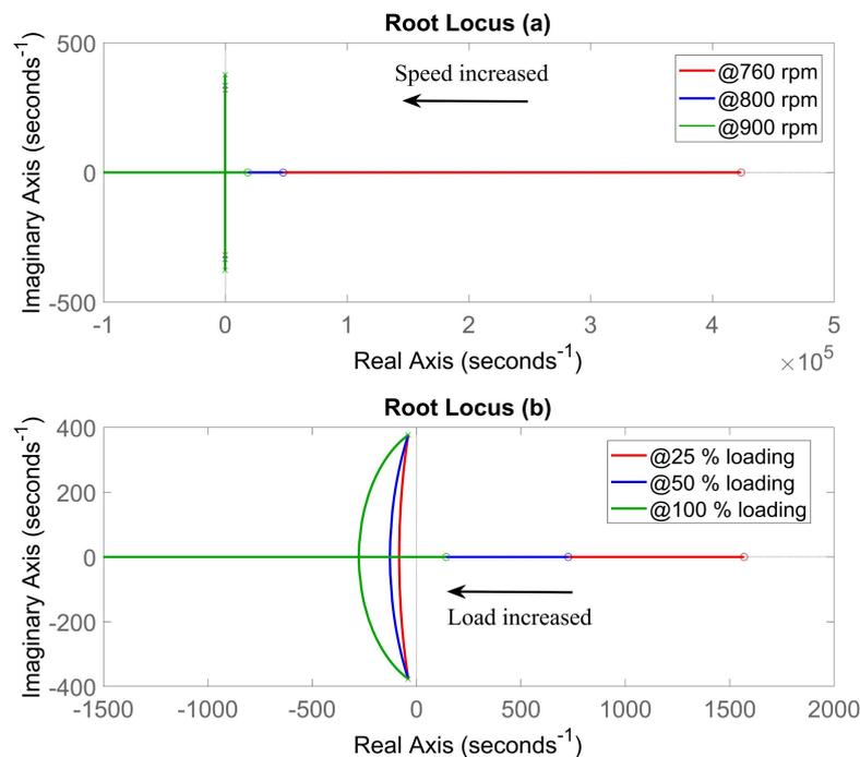
**Figure 7.** Pole zero movement for starter mode: (a) speed value at 760, 800, and 900 rpm at no load (b) load value at 25, 50, and 100 % of rated torque at 900 rpm.
