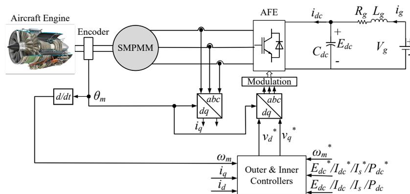
Figure 1. PMM based S/G system connected with AFE topology.
