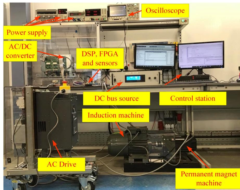
**Figure 16.** Layout of the experimental rig.
