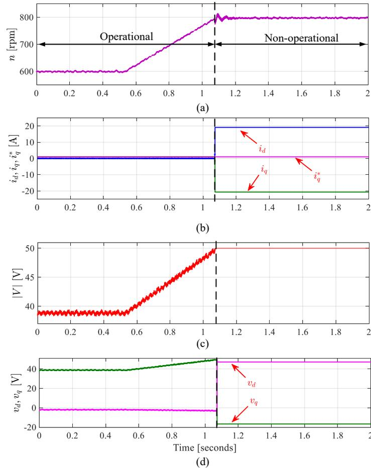
**Figure 17.** Experimental results of speed changes from 600 to 800 rpm using VVB method: (a) Speed, (b)  $dq$  currents, (c) Voltage magnitude and (d)  $dq$  voltages references sent to PWM modulator.
