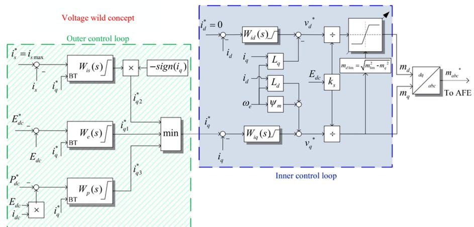
Figure 4. Variable Voltage Bus control strategy of PMM [14].
