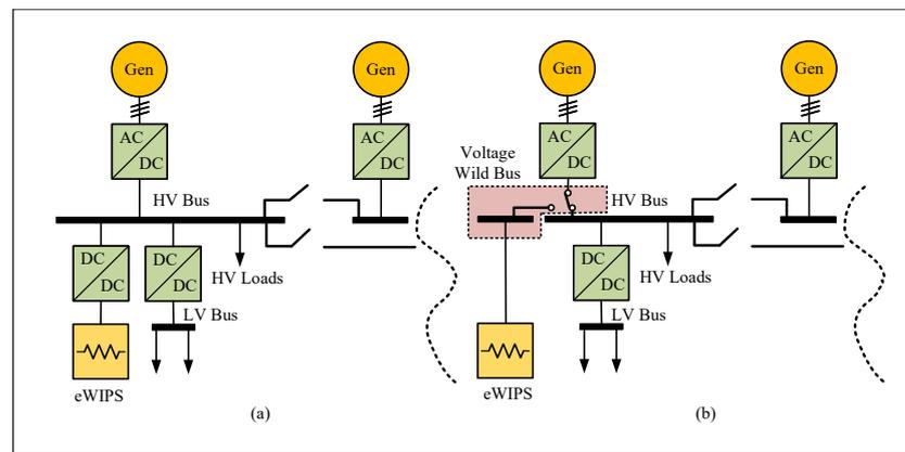
Figure 3. (a) Integration of WIPS in existing MEA EPS architectures. (b) Suggested integration [14].
