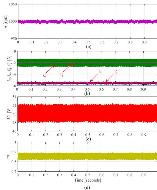
**Figure 25.** Experimental results of steady-state values for generating mode at speed 1000 rpm: (a) Speed, (b)  $dq$  currents, (c) Voltage magnitude and (d) Modulation index.
