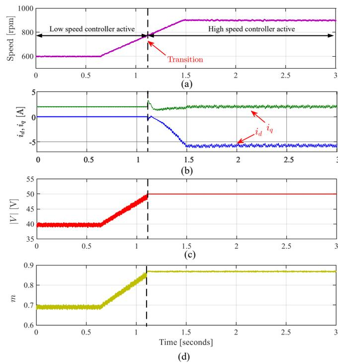
**Figure 19.** Experimental results of speed changes from 600 to 900 rpm using the proposed method: (a) Speed, (b)  $dq$  currents, (c) Voltage magnitude, and (d) Modulation index.
