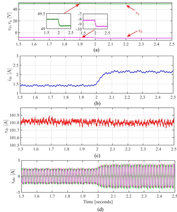
**Figure 24.** Experimental results of  $i_q^*$  changes from 2 to 3 A at 800 rpm using the proposed method: (a)  $dq$  voltages references sent to PWM modulator, (b) DC current, (c) DC bus voltage, (d) AC currents.
