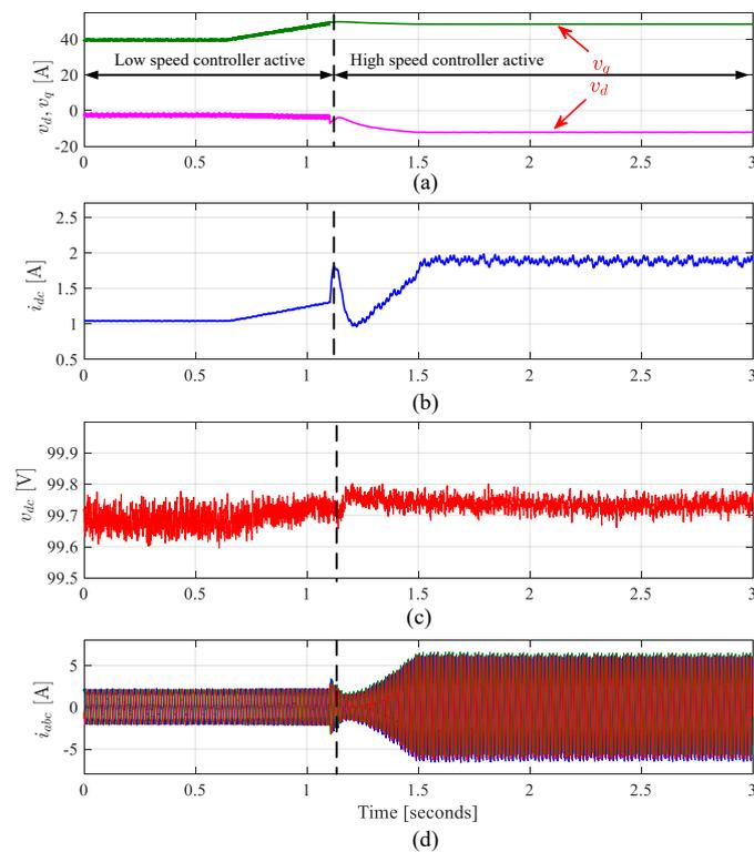
**Figure 20.** Experimental results of speed change from 600 to 900 rpm using the proposed method: (a)  $dq$  voltages references sent to PWM modulator, (b) DC current, (c) DC bus voltage, (d) AC currents.
