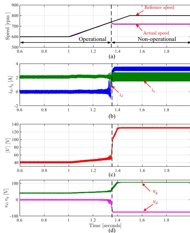
**Figure 5.** Time response of VVB control scheme in the starter mode: (a) Speed, (b)  $dq$  currents, (c) Voltage magnitude and (d)  $dq$  voltages.
