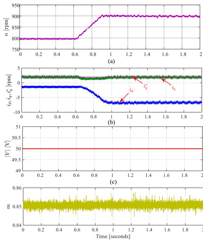
**Figure 21.** Experimental results of speed changes from 800 to 900 rpm using the proposed method: (a) Speed, (b)  $dq$  currents, (c) Voltage magnitude, and (d) Modulation index.
