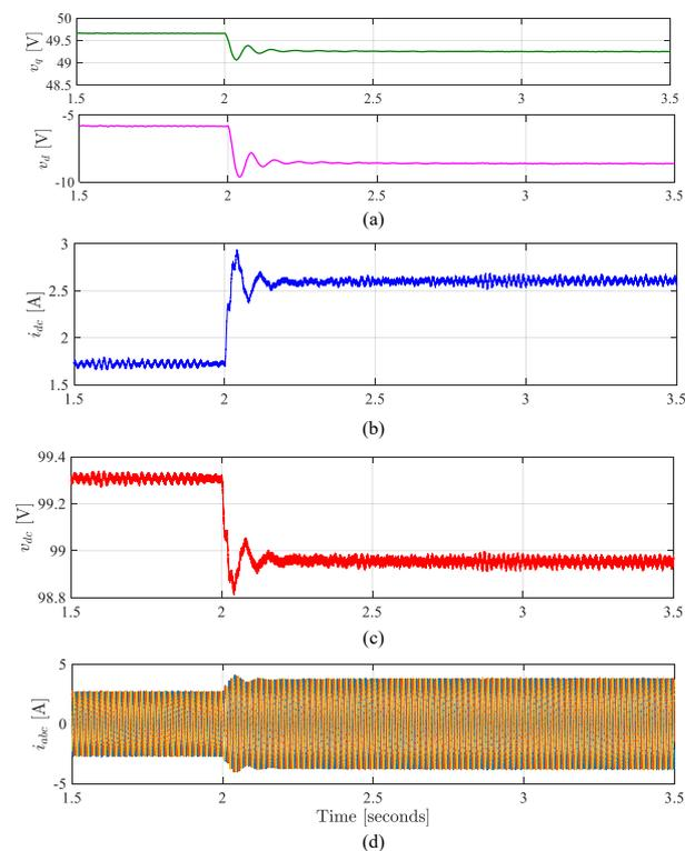
**Figure 13.** Simulation results of starter mode in FW with load change from 2 to 3 N-m at 800 rpm: (a)  $dq$  voltages references sent to PWM modulator, (b) DC current, (c) DC bus voltage, and (d) AC currents.
