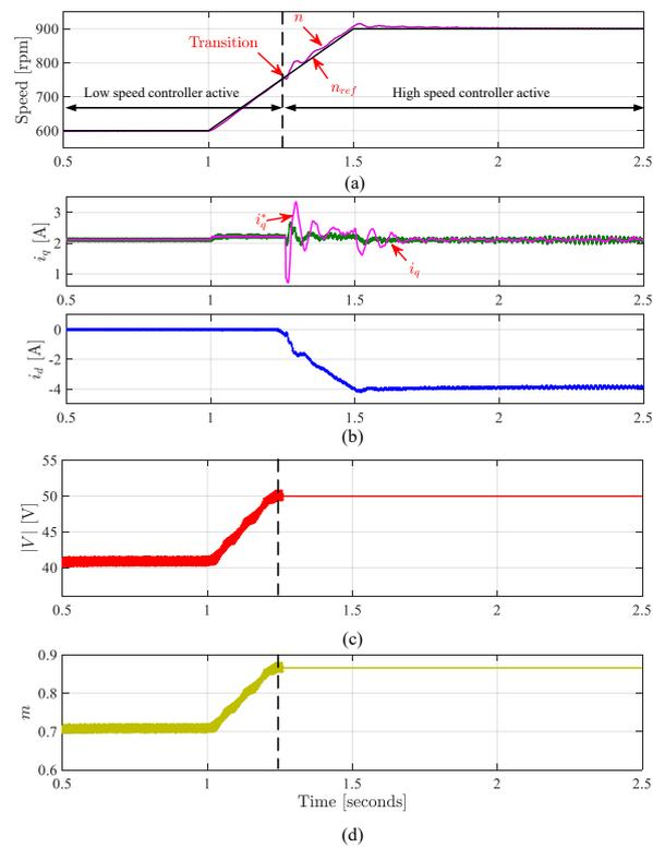
**Figure 10.** Simulation results of starter mode with speed change from 600 to 900 rpm, using the proposed method: (a) Speed, (b)  $dq$  currents, (c) Voltage magnitude, and (d) Modulation index.
