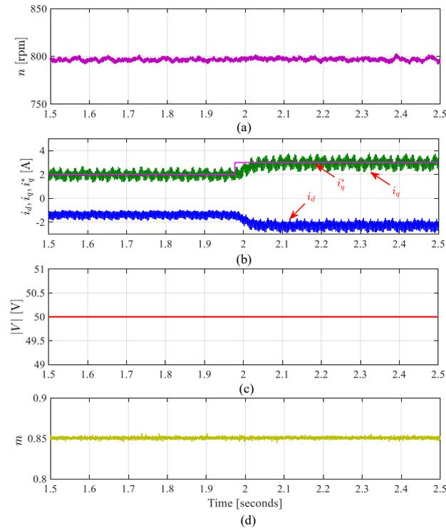
**Figure 23.** Experimental results of  $i_q^*$  changes from 2 to 3 A at 800 rpm using the proposed method: (a) Speed, (b)  $dq$  currents, (c) Voltage magnitude, and (d) Modulation index.
