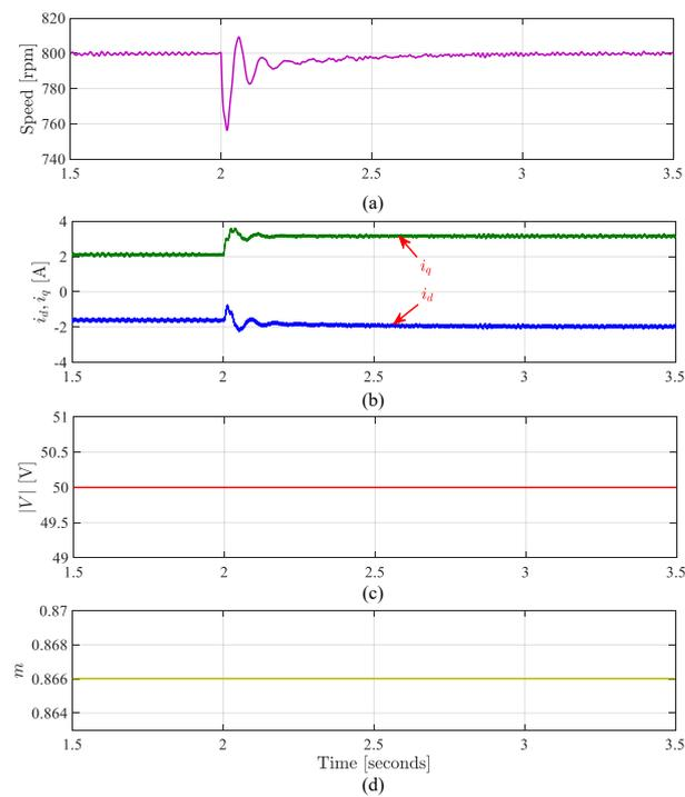
**Figure 12.** Simulation results of starter mode in FW with load change from 2 to 3 N-m at 800 rpm: (a) Speed, (b)  $dq$  currents, (c) Voltage magnitude, and (d) Modulation index.
