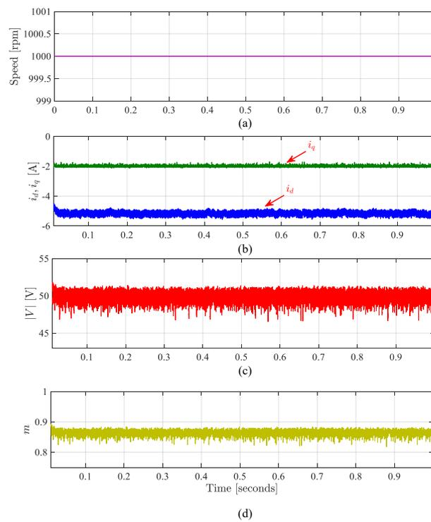
**Figure 14.** Simulation results of generation mode in FW with  $i_q^* = -2$  A at 1000 rpm: (a) Speed, (b)  $dq$  currents, (c) Voltage magnitude and (d) Modulation index.
