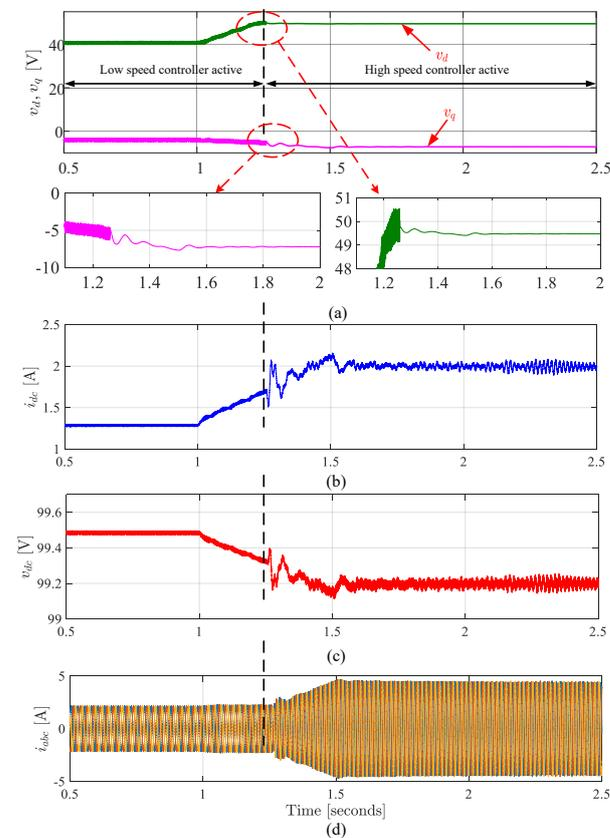
**Figure 11.** Simulation results of starter mode with speed change from 600 to 900 rpm using the proposed method: (a)  $dq$  voltages references sent to PWM modulator, (b) DC current, (c) DC bus voltage, (d) AC currents.
