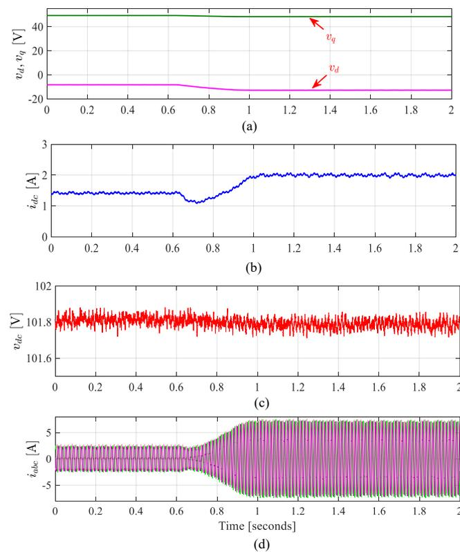
**Figure 22.** Experimental results of speed changes from 800 to 900 rpm using the proposed method: (a)  $dq$  voltages references sent to PWM modulator, (b) DC current, (c) DC bus voltage, (d) AC currents.
