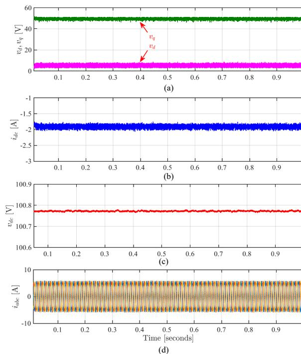
**Figure 15.** Simulation results of generation mode in FW with  $i_q^* = -2$  A at 1000 rpm: (a)  $dq$  voltages references sent to PWM modulator, (b) DC current, (c) DC bus voltage, and (d) AC currents.
