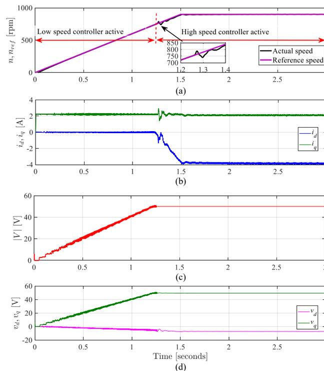
**Figure 9.** Time response for start-up mode from standstill to 900 rpm using the proposed method: (a) Speed, (b)  $dq$  currents, (c) Voltage magnitude and (d)  $dq$  voltage references sent to PWM modulator.
