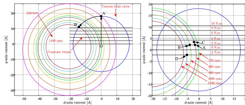
Figure 2. Voltage and current limit circles @  $|V_{max}| = 50$  V, (left): Normal circles and (right): Zoom in of circles.
