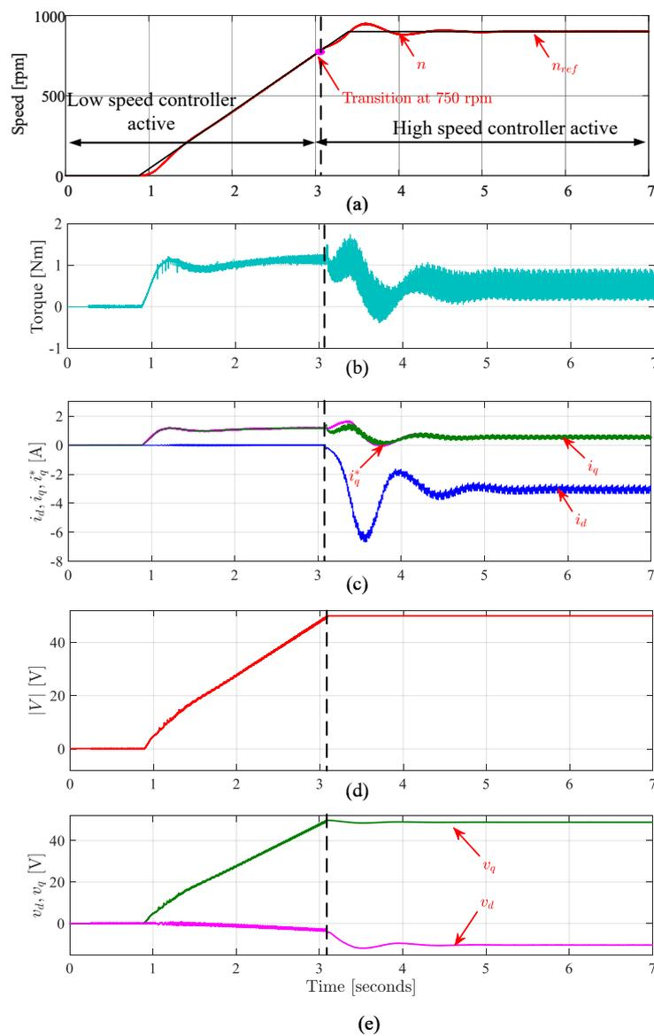
**Figure 18.** Experimental results of start-up mode using the proposed method from standstill to 900 rpm for the test bench AC drive system: (a) Speed, (b) Electromagnetic torque (c)  $dq$  currents, (d) Voltage magnitude and (e)  $dq$  voltages references sent to PWM modulator.
