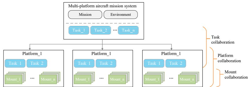
Figure 2. The block diagram of the MPAMS organization.
