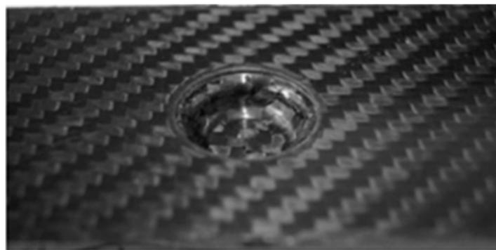
**Figure 5.** Corrugation formed into a thermoset matrix woven composite laminate [24].
