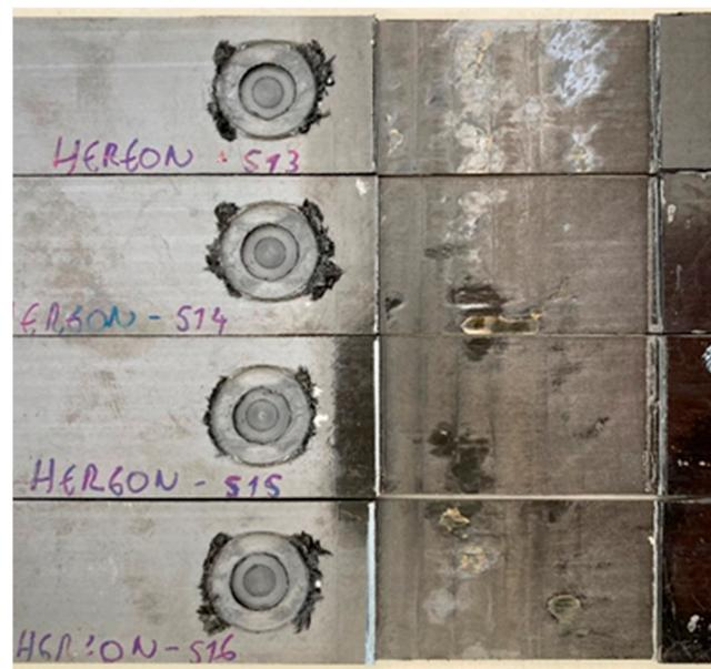
**Figure 10.** The RFSSW feature installed as CAF on crack lap shear specimens.
