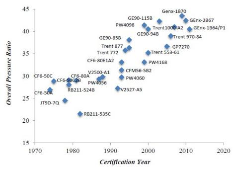
**Figure 1.** An overview of engine pressure ratio development over the years [18] (reprinted with permission).
