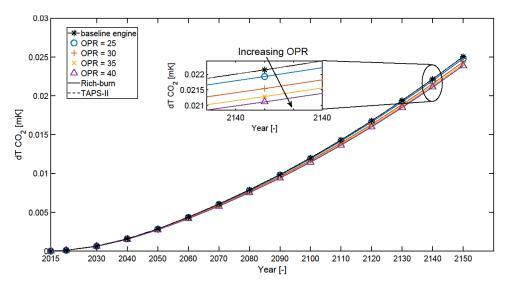
Figure 18. Temporal evolution of the temperature response due to  $CO_2$  emissions (dT  $CO_2$ ) for baseline engine (dotted-asterisk line) and the OPR range from 25 to 40. The trends are shown for both combustor technologies (in this case, they result in identical trendlines). The response due to the different configurations is also shown for the year 2140.
