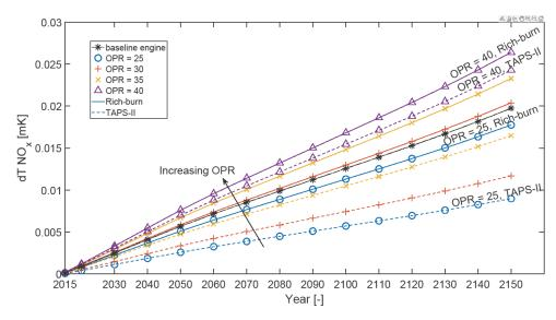
Figure 19. Temporal evolution of the temperature response due to  $NO_x$  emissions (enhancement effects due to  $O_3$  production and diminishing effects due to  $CH_4$  and PMO) for baseline engine (dotted asterisk line) and the OPR range from 25 to 40. Solid lines represent rich-burn configurations, whereas dashed lines represent TAPS-II configurations.
