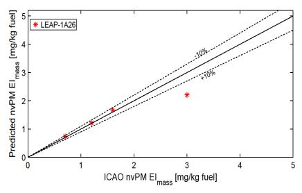
**Figure 7.** Comparison of the model—predicted nvPM  $EI_{mass,SLS}$  (Equation (14)) with ICAO—provided nvPM under SLS conditions for one LEAP—X model (total four points) for the TAPS—II combustor. The solid dashed line is used as a reference to measure the accuracy of the model, with the dashed lines representing a  $\pm 10\%$  deviation.
