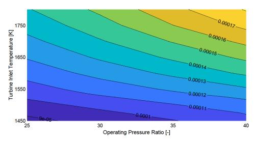
**Figure 16.** Cruise nvPM number of the fleet with varying OPR and TIT for the TAPS-II combustor configurations, normalized to the baseline, which is  $1.4 \times 10^{20}$  (#nvPM) (Table 1).
