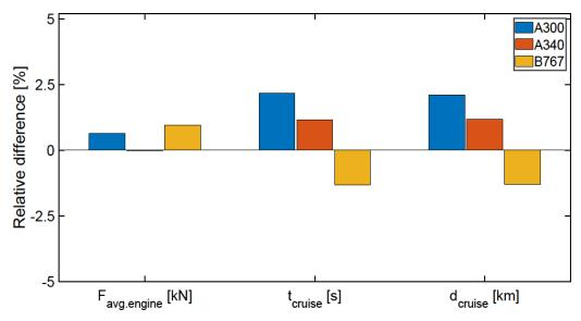
**Figure 3.** Relative difference of key aircraft performance parameters calculated by the in–house model with respect to PIANO–X output.
