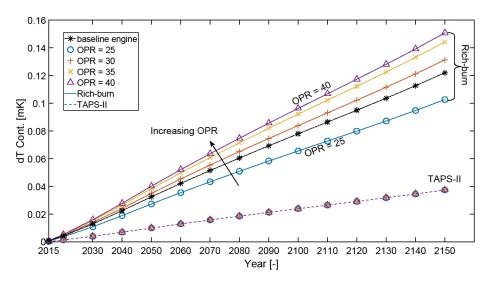
**Figure 20.** Temporal evolution of the temperature response due to contrail effects (dT Cont.) for baseline engine (dotted asterisk line) and the OPR range from 25 to 40. Solid lines represent rich-burn configurations, whereas dashed lines represent TAPS-II configurations.
