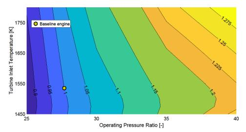
**Figure 14.** ATR<sub>100</sub> with varying OPR and TIT for the rich-burn combustor configurations, normalized to the baseline (yellow circle), which is 0.085 mK (Table 1).
