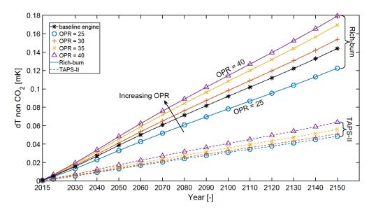
**Figure 21.** Temporal evolution of the temperature response due to the non- $CO_2$  emissions (dT  $NO_X$ ,  $H_2O$ , and contrails) for baseline engine (dotted-asterisk line) and the OPR range from 25 to 40. Solid lines represent rich-burn configurations, whereas dashed lines represent TAPS-II configurations.
