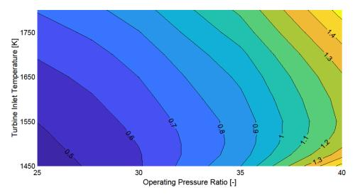
**Figure 15.** Cruise  $NO_X$  emissions of the fleet with varying OPR and TIT for the TAPS-II combustor configurations, normalized to the baseline, which is 3.11  $t(NO_2)$  (Table 1).
