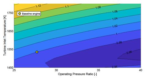
**Figure 11.** Cruise fuel consumption of the fleet with varying OPR and TIT for the rich-burn combustor configurations, normalized to the baseline (yellow circle), which is 279.28 t(fuel) (Table 1).
