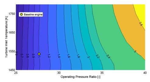
**Figure 13.** Cruise nvPM number of the fleet with varying OPR and TIT for the rich-burn combustor configurations, normalized to the baseline (yellow circle), which is  $1.4 \times 10^{20}$  (#nvPM) (Table 1).
