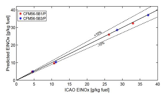
**Figure 4.** Comparison of the model–predicted EINO<sub>x</sub> (Equation (7)) with the ICAO–provided EINO<sub>x</sub> under SLS conditions for two CFM56 models (total eight points) for the rich–burn combustor. The solid dashed line is used as a reference to measure the accuracy of the model, with the dashed lines representing a  $\pm 10\%$  deviation.
