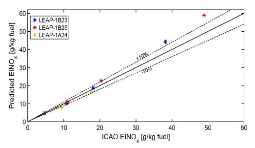
**Figure 6.** Comparison of the model–predicted EINO<sub>x</sub> (Equation (13)) with the ICAO–provided EINO<sub>x</sub> under SLS conditions for three LEAP models (total twelve points) for the TAPS–II combustor. The solid dashed line is used as a reference to measure the accuracy of the model, with the dashed lines representing a  $\pm 10\%$  deviation.
