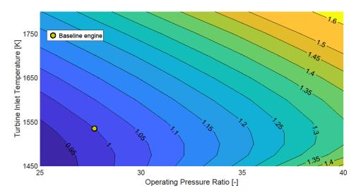
**Figure 12.** Cruise  $NO_x$  emissions of the fleet with varying OPR and TIT for the rich-burn combustor configurations, normalized to the baseline (yellow circle), which is 3.11 t( $NO_2$ ) (Table 1).
