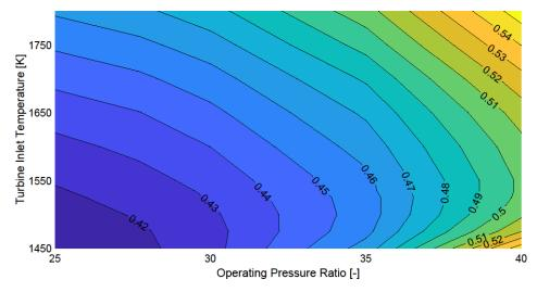
**Figure 17.** ATR $_{100}$  with varying OPR and TIT for the TAPS-II combustor configurations, normalized to the baseline, which is 0.085 mK (Table 1).
