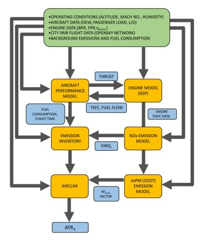
**Figure 2.** The overview of the modeling chain implemented in this research. The contents in green at the top represent the various boundary/operating conditions, those in yellow represent the various models, and those in blue represent the relevant parameters and outputs of interest.
