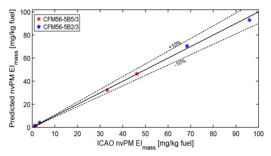
**Figure 5.** Comparison of the model–predicted nvPM  $EI_{mass,SLS}$  (Equation (10)) with ICAO–provided nvPM under SLS conditions for two CFM56 models (total eight points) for the rich–burn combustor. The solid dashed line is used as a reference to measure the accuracy of the model, with the dashed lines representing a  $\pm 10\%$  deviation.
