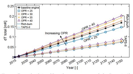
**Figure 22.** Temporal evolution of the total temperature response for baseline engine (dashed asterisk line) and an OPR ranging from 25 to 40. Solid lines represent rich-burn configurations, whereas dashed lines represent TAPS-II configurations.
