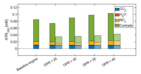
**Figure 23.** Comparison of the ATR<sub>100</sub> for each of the six species for the lowest fuel consumption configurations with changing OPR. The trends for the rich burn combustor are shown in solid, whereas those for the TAPS–II combustor are shown as hatched.
