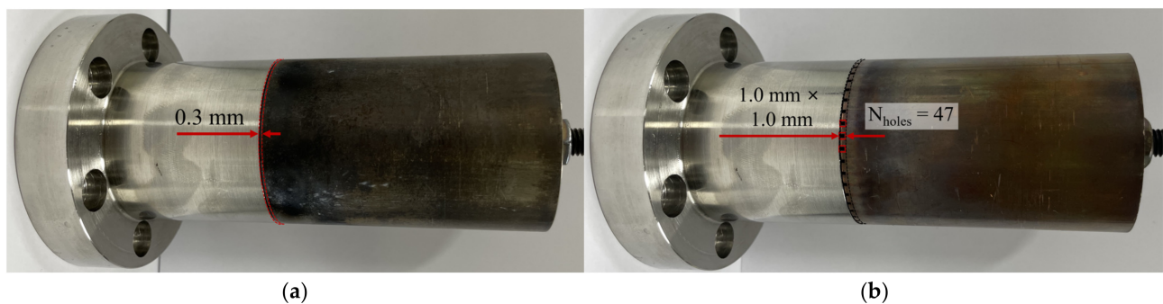
Figure 5. Injector of the RDE experimental model: (a) SFI, 0.3 mm in width; (b) RHFI consisting of 47 holes with a square shape of 1.0 mm 2 .
