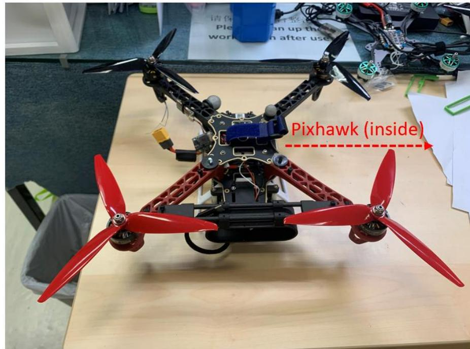
**Figure 3.** The F330 UAV set up.
