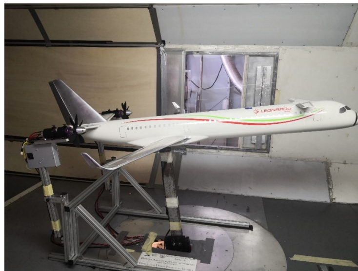
Figure 16. Aircraft complete configuration with electric motors.
