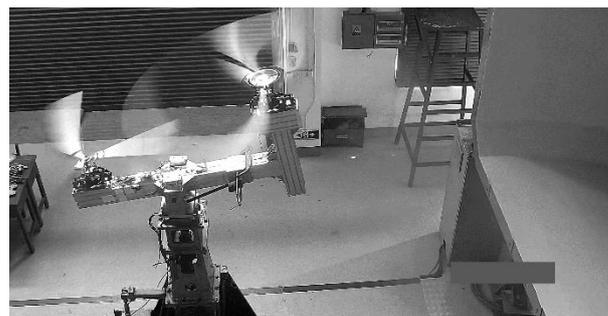
**Figure 5.** Tandem rotor test of autorotation in forward flight.
