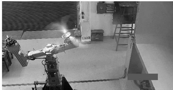
**Figure 4.** Isolated rotor test of autorotation in forward flight.
