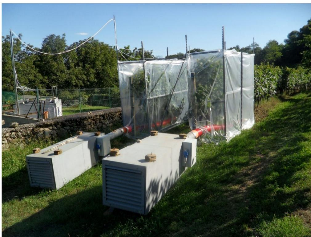
**Figure 1.** View of two of the four open top chambers enclosing grapevine plants on the chosen vineyard in Angera. The chambers were fed with air which was ambient or charcoal-filtered.
