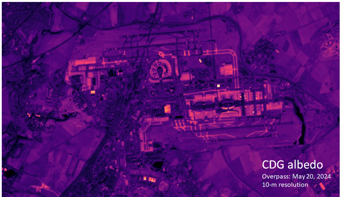
Figure A1. Broad-band albedo derived from 10-m Sentinel-2 reflectance data.
