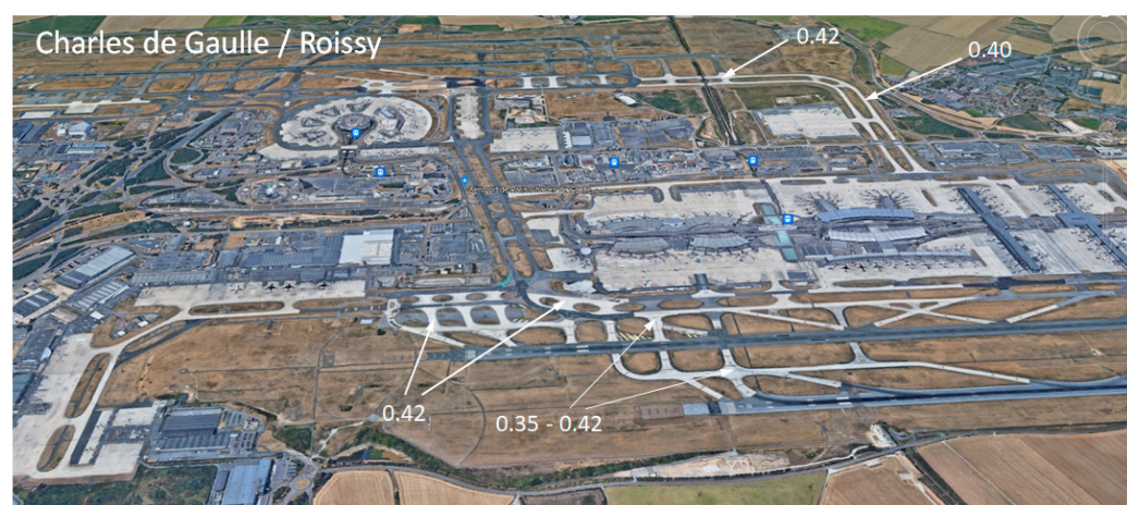
Figure 5. Broad-band (10 m resolution) albedo computed from Sentinel-2 for Charles de Gaulle airport (CDG).
