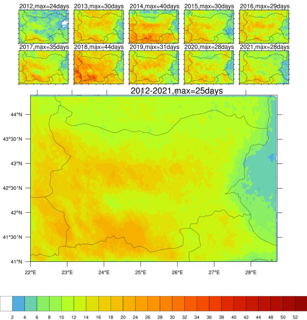
**Figure 10.** Annual spatial (on a grid of  $0.05 \times 0.05$  deg) distribution of days with flashes (number of days with flashes per year) according to ATDnet during 2012, 2013, 2014, 2015, 2016, 2017, 2018, 2019, 2020, and 2021, and the yearly average for the whole period 2012–2021.
