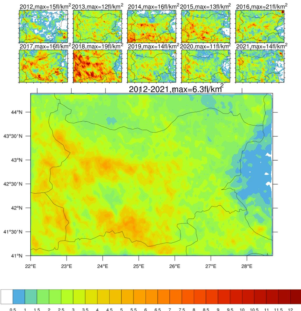
**Figure 9.** Annual spatial (on a grid of  $0.05 \times 0.05$  deg) distribution of flash density (number of flashes per  $\text{km}^2$  per year), according to ATDnet during 2012, 2013, 2014, 2015, 2016, 2017, 2018, 2019, 2020, and 2021, and the yearly average for the whole period 2012–2021.
